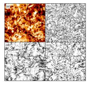
FIG. 2 (color online). (a) The modulus of the pressure gradient, giving the main contribution to fluid acceleration, on a slice  $512 \times 512 \times 4$ . B/W code low and high intensity, respectively. Particle positions in the same slice are shown for (b)  $S_{\eta} = 0.16$ , (c) 0.80, and (d) 3.30. Note the presence of voids with sizes much larger than the dissipative scale.
