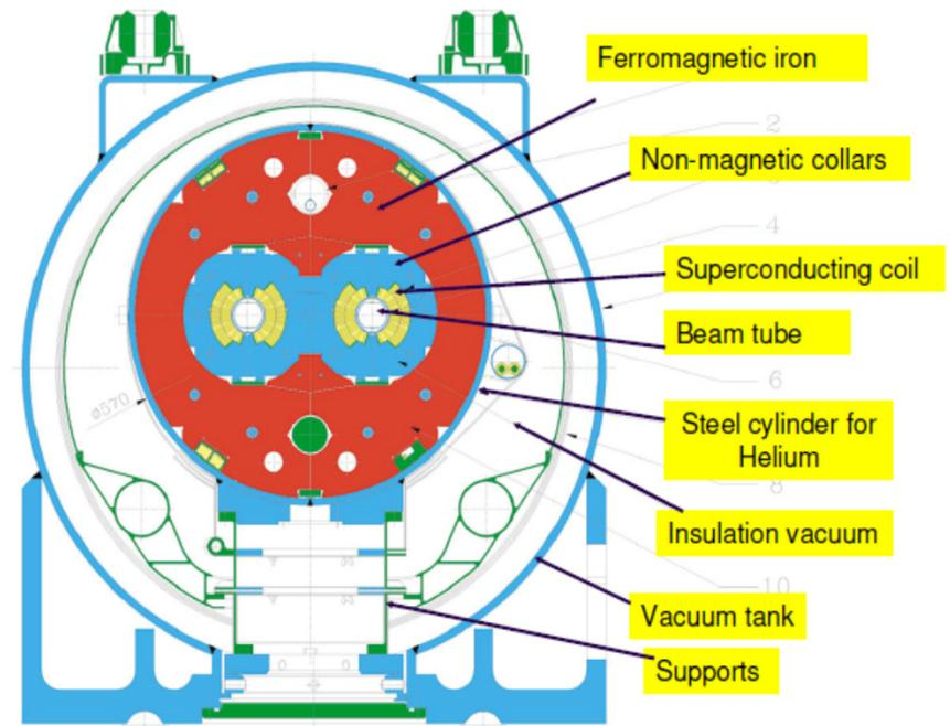
Weight (magnet + cryostat) ~ 30 tons, length 15 m
