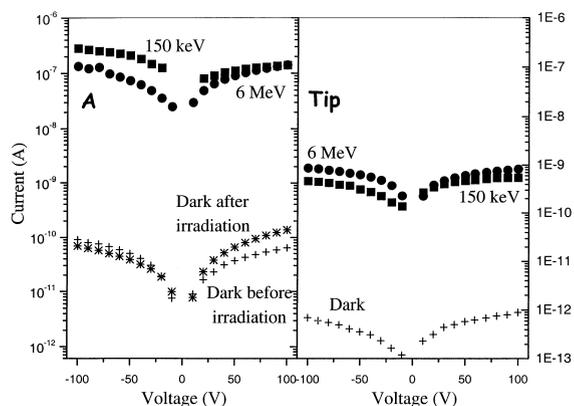
Fig. 3. Sensitivity of the two diamond detectors as a function of applied bias voltage under dark conditions and under X-rays generated by a continuous X-ray source (150 kV<sub>p</sub>) and linear accelerator (6 MeV).
