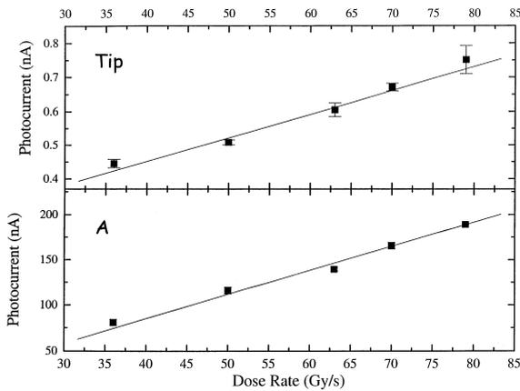
Fig. 4. Photocurrents measured at 100 V bias as a function of dose rate. The X-ray tube voltage is 150 kV.
