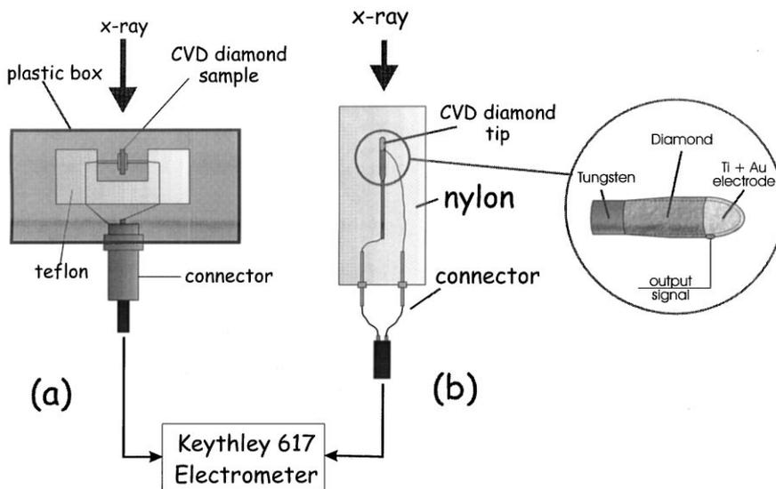
Fig. 1. Scheme of the experimental set-up for the two diamond samples used as X-ray dosimeters.
