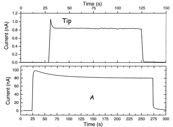
Fig. 6. Photocurrents measured during a 6 MeV beam switch-on-switch-off cycle at 100 V bias as a function of time.
