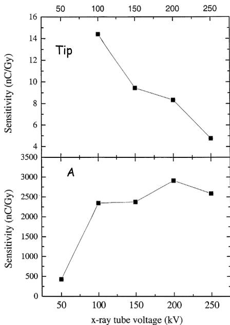
Fig. 5. Sensitivities as functions of X-ray tube peak voltage. The X-ray tube current is 10 mA.
