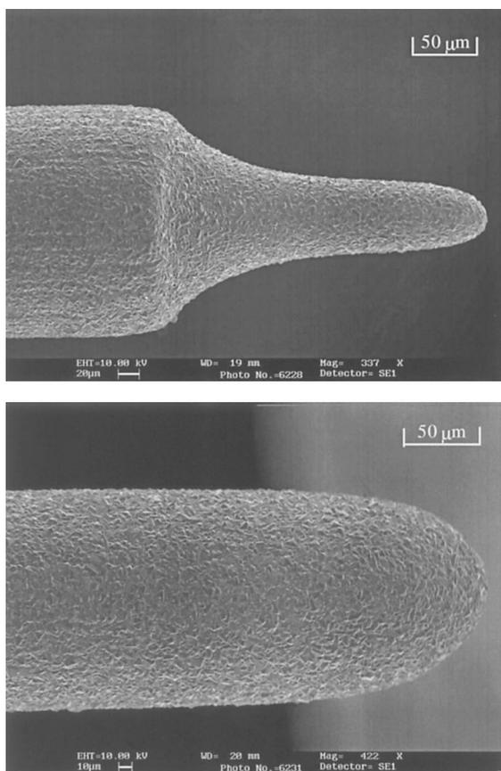
Fig. 2. Scanning electron microscopy photographs of two CVD diamond films grown at the end of three 200  $\mu\text{m}$  tungsten wires etched by the electrochemical method described in Ref. [3] under different etching conditions.
