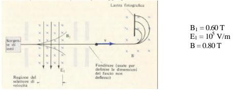
a) Find the relation between  $\mathbf{v}$ ,  $\mathbf{B}_1$  and  $\mathbf{E}_1$  and compute the velocity of the filtered ions. Ions with the same velocity are then deflected by a magnetic field  $\mathbf{B}$  on a circular trajectory of radius R according to their mass m and strike a photographic plate after one-half a revolution.
