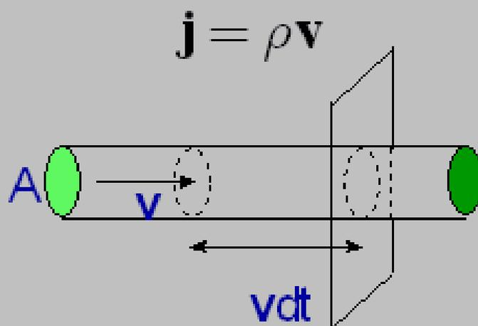
$$dQ = \rho dV = \rho \underbrace{A \cdot v}_{\substack{\text{velocita'} \\ \times \\ \text{area perp.}}} dt$$
