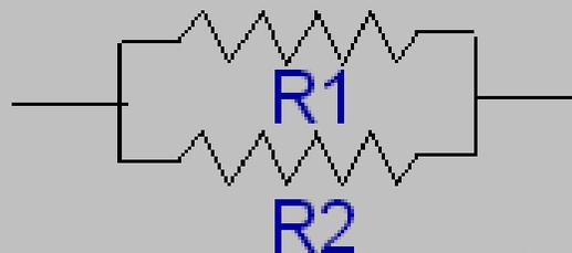
$$i = i_1 + i_2 = \frac{V}{R_1} + \frac{V}{R_2} = V \left( \frac{1}{R_1} + \frac{1}{R_2} \right)$$
