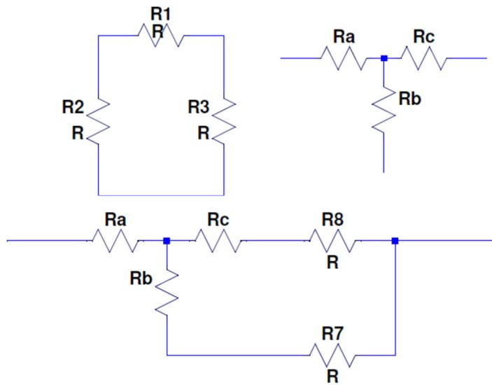
$$R_{10} = R_a + (R_c + R_8) \parallel (R_b + R_7)$$
