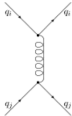
Figure 1: Feynman diagram for q_i q_j \rightarrow q_i q_j, i \neq j
