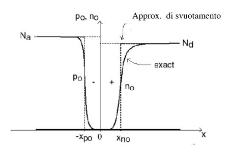
$$\begin{aligned} x < -x_{p0}: & p_0(x) = N_A, n_0(x) = \frac{n_i^2}{N_A} \\ -x_{p0} < x < 0: & p_0(x), n_0(x) \ll N_A \\ 0 < x < +x_{n0}: & n_0(x), p_0(x) \ll N_D \\ x > +x_{n0}: & n_0(x) = N_D, p_0(x) = \frac{n_i^2}{N_D} \end{aligned}$$
