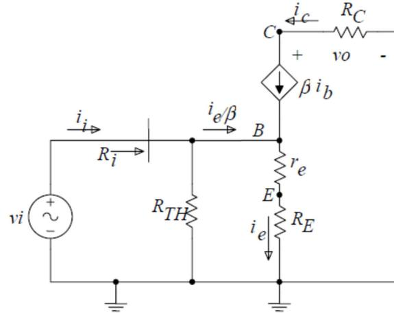
$$R_i = \frac{v_i}{i_i} = R_{TH} \parallel (1 + \beta)(r_e + R_E)$$
