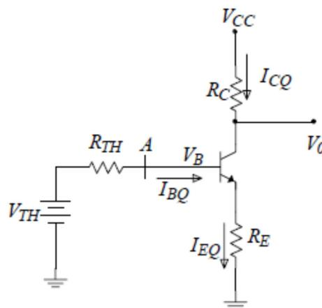
$$R_{TH} = \frac{R_1 R_2}{R_1 + R_2}, V_{TH} = V_{CC} \frac{R_2}{R_1 + R_2}$$
