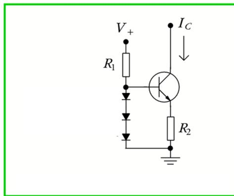
$$V_{diodi} \simeq 1.8V \rightarrow V_2 \simeq 1.2V \rightarrow I_E = \frac{V_{diodi} - V_{BE}}{R_2} \simeq \frac{1.2}{R_2} \simeq I_C$$
