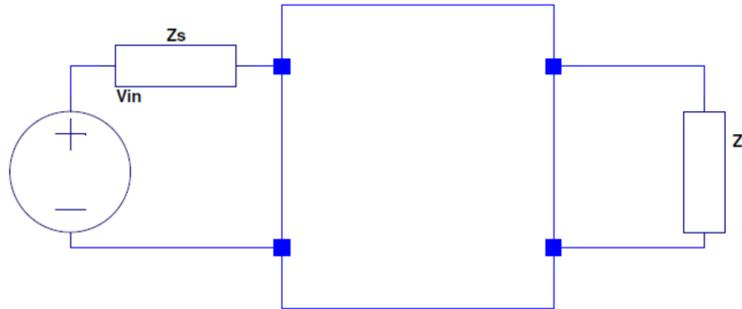
$$\begin{cases} v_1 = z_{11}i_1 + z_{12}i_2 \\ -Z_L i_2 = z_{21}i_1 + z_{22}i_2 \end{cases} \rightarrow \begin{cases} v_1 = z_{11}i_1 + z_{12}i_2 \\ 0 = z_{21}i_1 + (z_{22} + Z_L)i_2 \end{cases}$$
