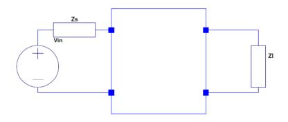
$$\begin{cases} v_{1} = z_{11}i_{1} + z_{12}i_{2} \\ -Z_{L}i_{2} = z_{21}i_{1} + z_{22}i_{2} \end{cases} \rightarrow \begin{cases} v_{1} = z_{11}i_{1} + z_{12}i_{2} \\ 0 = z_{21}i_{1} + (z_{22} + Z_{L})i_{2} \end{cases}$$
