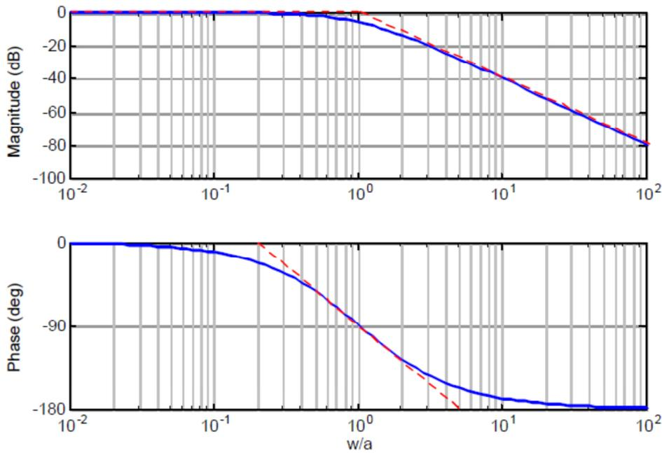
$$H(s) = \frac{\omega_n^2}{s^2 + 2\zeta\omega_n s + \omega_n^2} \quad \text{Poli complessi coniugati}$$
