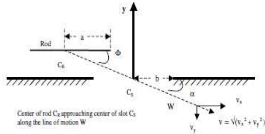
Figure 5. Initial conditions of the rod-slot problem.
