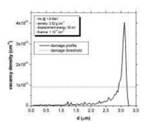
FIG. 1. TRIM Monte Carlo simulations of the damage density profile induced in diamond by 1.8 MeV He<sup>+</sup> at a fluence of  $1 \times 10^{17}$  cm<sup>2</sup> (solid line), together with the graphitization threshold (dashed line).
