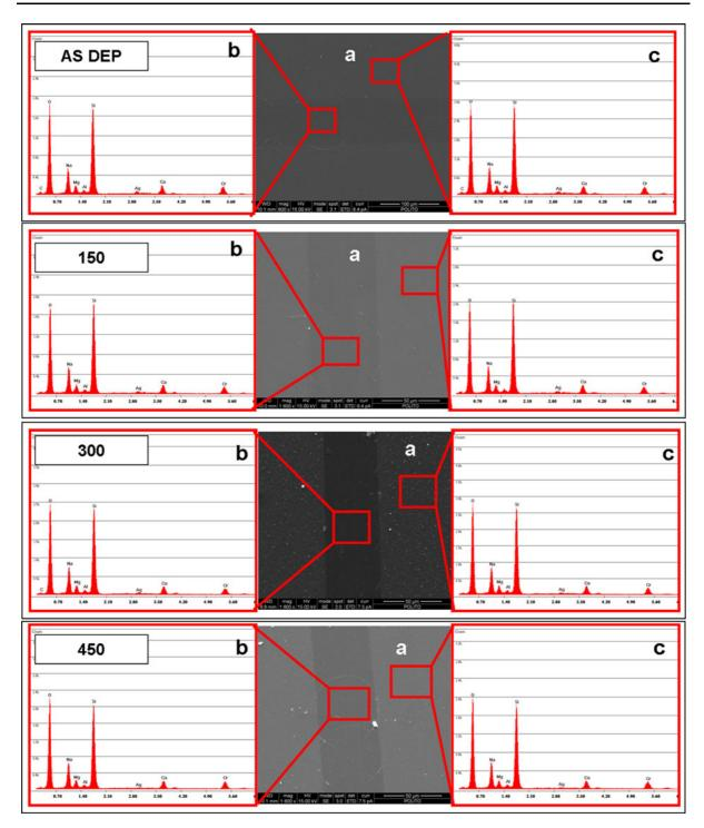
Fig. 10 Scratch tracks on silver nanocluster/silica composite coatings on soda-lime glasses as-deposited and after thermal treatments: SEM images (a) and EDS analyses in the track (b) and out of it (c)
