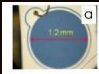
Hamamatsu S5821 p-i-n diode
