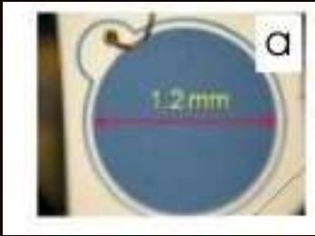
Hamamatsu S5821 p-i-n diode
