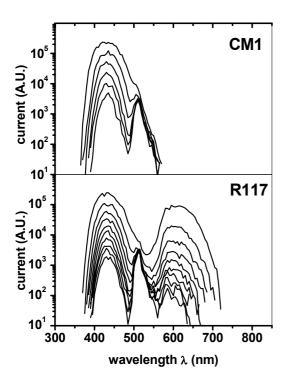
Fig. 1 - IBIL spectra of CVD diamond samples CM1 and R117 as recorded at increasing times. IBIL intensity continuously decreases. Each spectrum corresponds to about  $10^{15}$  p/cm<sup>2</sup> of proton dose over a surface area of 0.5 x 0.5 mm<sup>2</sup>. Sample R117 is characterized by a poorer charge carrier collection efficiency with respect to the sample CM1.
