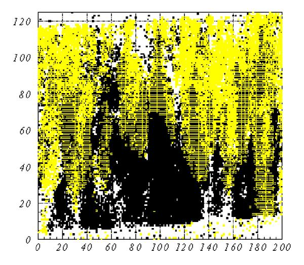
Superimposed IBIC ( yellow ) and IBIL ( black ) maps obtained irradiating the cross section of a CVD diamond film (400  $\mu m$  x 800  $\mu m$ ). Growth side is at the top, substrate side is at the bottom.
