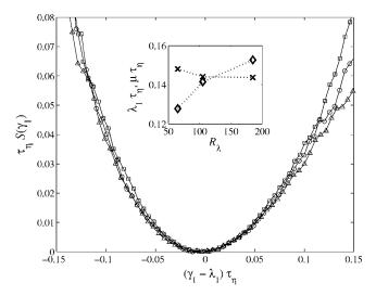
FIG. 3. Cramér function  $S(\gamma_1)$  for fluid tracers for  $R_{\lambda}$ =65 (squares), 105 (circles), and 185 (triangles). Inset: Lyapunov exponent  $\lambda_1$  (crosses) and reduced variance  $\mu = T\sigma^2$  (diamonds) as a function of  $R_{\lambda}$ .
