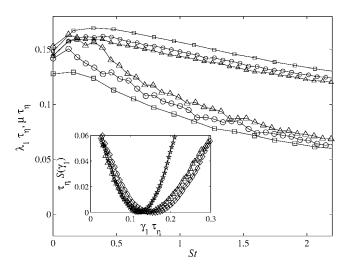
FIG. 4. Mean value  $\lambda_1$  (small symbols) and reduced variance  $\mu$  (large symbols) of the FTLE as a function of the Stokes number, for  $R_{\lambda}$ =65 (squares),  $R_{\lambda} = 105$  (circles), and  $R_{\lambda} = 185$  (triangle). Inset: Cramér function  $S(\gamma_1)$  for  $R_{\lambda} \approx 185$ , and various values of the Stokes number: St=0 (triangles), St=0.32 (diamonds), and St=2.19 (stars).
