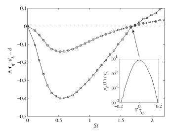
FIG. 2. Lyapunov dimension  $d_{\lambda}$  (squares) and volume growth rate  $\Lambda$  $=\sum_{i=1}^{3}\lambda_{i}$  (circles) as a function of Stokes number  $(R_{\lambda}=185)$ . Inset: PDF of the finite-time volume growth rate  $\Gamma(T)$  for  $T \approx 80\tau_n$ .
