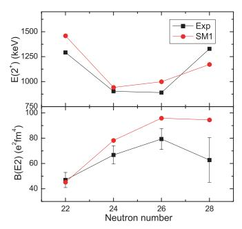
FIG. 5. (Color online) The systematics of experimental  $2_1^+$  energies and  $B(E2; 2_1^+ \to 0_{\rm g.s.}^+)$  values in even-A sulfur isotopes for neutron numbers in the range  $22 \le N \le 28$ .
