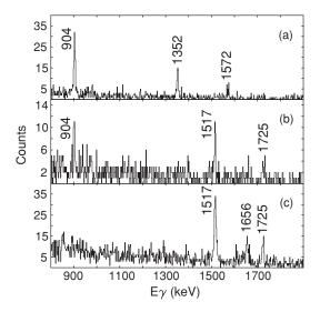
FIG. 2. Doppler-corrected partial  $\gamma$ -ray spectra corresponding to gates set in regions a to c of the mass spectrum of Fig. 1. (top) Spectrum corresponds to region a of the mass spectrum and shows  $\gamma$ -ray transitions within the  $^{40}$ S yrast decay sequence. (bottom) Spectrum dominated by yrast transitions in  $^{39}$ S. (middle) Spectrum corresponds to a gate set between the mass 39 and 40 peaks of Fig. 1. See text for details.
