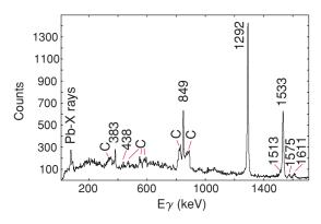
FIG. 3. (Color online) The partial  $\gamma$ -ray spectrum from the decay of excited states of  $^{38}$ S populated in this article. Peaks labeled "C" correspond to the decay of targetlike fragments. The spectrum illustrates the population of yrast states in binary grazing reactions.
