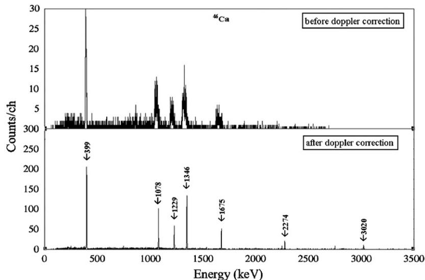
Fig. 9. Comparison between uncorrected and Doppler-corrected spectra for the  $^{46}\text{Ca}$  isotope.
