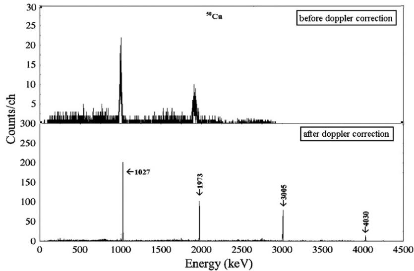
Fig. 10. Comparison between uncorrected and Doppler-corrected spectra for the  $^{50}\text{Ca}$  isotope.
