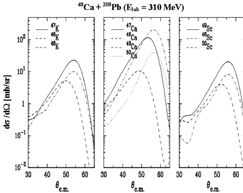
Fig. 6. Differential cross-sections and angular distributions calculated with the Grazing code for the  $^{48}\text{Ca} (310 \text{ MeV}) + ^{208}\text{Pb}$  reaction. Data are calculated in the centre-of-mass reference frame.
