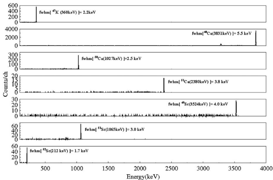
Fig. 5. Doppler-corrected peaks for the following ions:  $^{47}\text{K}$  (360 keV),  $^{48}\text{Ca}$  (3831.80 keV),  $^{50}\text{Ca}$  (1027 keV),  $^{51}\text{Ca}$  (2380 keV),  $^{49}\text{Sc}$  (3524 keV),  $^{51}\text{Sc}$  (1065 keV),  $^{52}\text{Sc}$  (212 keV).
