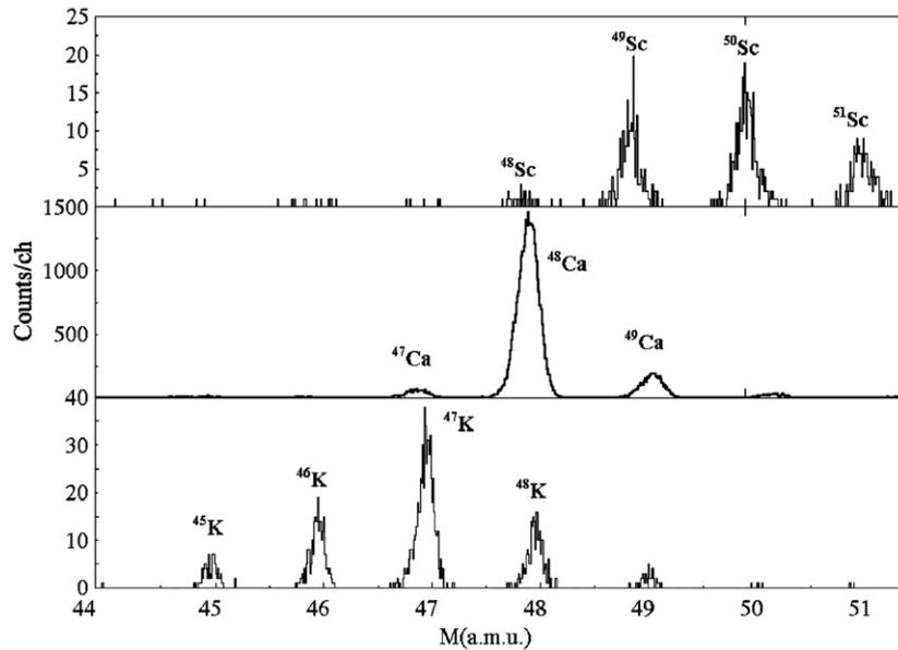
Fig. 4. The mass distributions of Sc, Ca, and K reaction products of the  $^{48}\text{Ca}+^{208}\text{Pb}$  reaction at PRISMA simulation.
