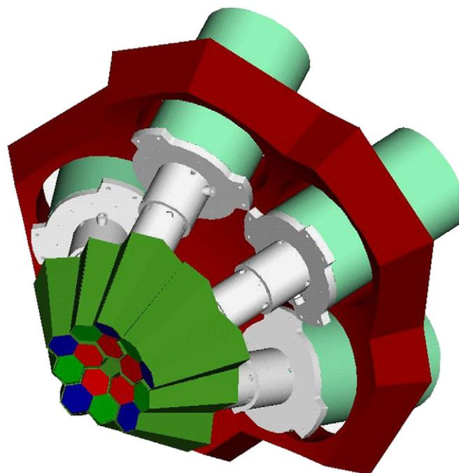
**Fig. 1.** Pictorial view of the AGATA Demonstrator Array, composed of 15 detectors arranged into five triple clusters.
